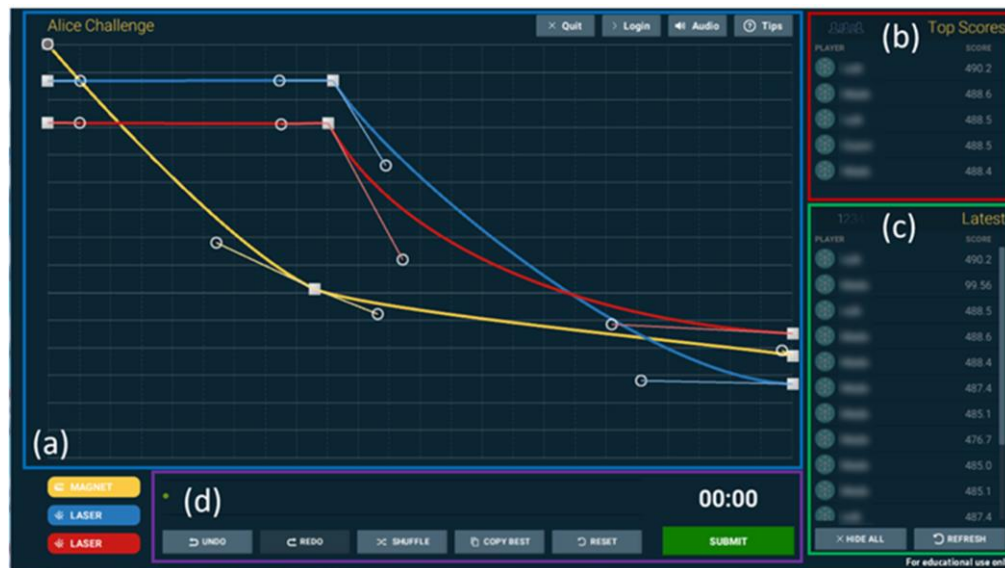
Figure 14. The interface for the Alice challenge, showing (a) the spline curves that the users could manipulate to control the time-dependent laser powers and magnetic field coil currents that controlled the final BEC atom number, (b) a top score list, (c) a list of the latest submissions and their scores and (d) a control toolbar, including the estimated wait time. Players could take any other player's solution (as shown in (b) and (c)) and modify it. Figure reproduced from 156 .
